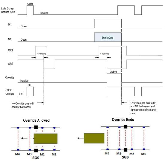
Figure 3. Muting Timing Diagram - T Configuration
