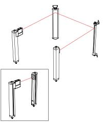
Figure 19. Optical alignment using the LAT-1-SGS
