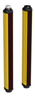
Banner's SGS Safety Grid System with Integral Muting is a two-piece, redundant, microprocessor-controlled, retroreflective optoelectronic "light grid". Standard models are available in 2 beam (500 mm beam spacing), 3 beam (400 mm beam spacing), or 4 beam (300 mm and 400 mm beam spacing) systems.
