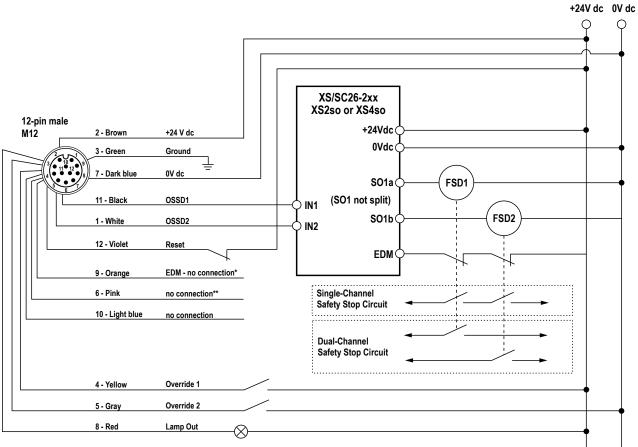
\* EDM Mode on the SGS Receiver must be set for No Monitoring
