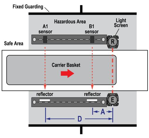
Figure 28. Exit Application with 1-Way Muting using two opposed-mode sensors
