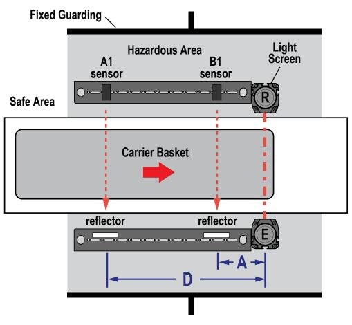
Figure 7. L Configuration-Uses two pairs of opposed-mode photoelectric sensors stationed on one side of the light curtain
