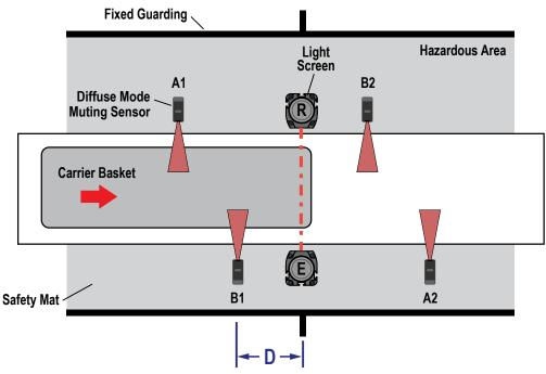
Figure 6. T Configuration-Uses two pairs of diffuse sensors
