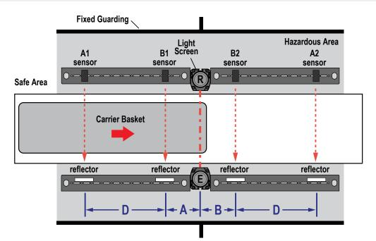
Figure 27. Entry/Exit Application using four pairs of opposed-mode photoelectric sensors for mute devices
