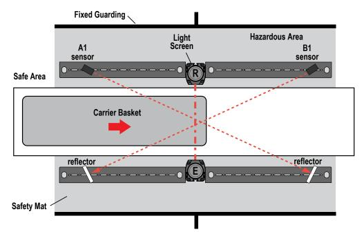
Figure 24. "X"-Pattern Entry/Exit system using two pairs of opposed-mode photoelectric muting devices
