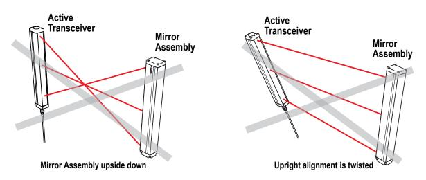
Figure 11. Examples of Incorrect Active Transceiver/Mirror Assembly Orientation
