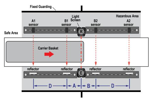
Figure 5. T Configuration – Uses four pairs of opposed-mode photoelectric sensors for mute devices
