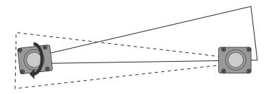
If the components are not aligned, the Last Couple and First Couple lights are on, the green status light is off, the red status light is on, and the 7-segment display shows an A.
