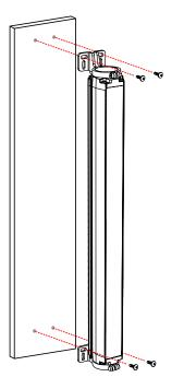
Figure 13. End-Mount Brackets
