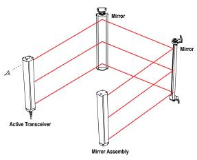
Figure 20. Corner Mirror Alignment
