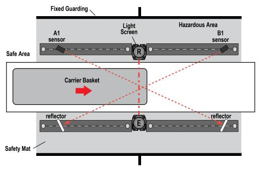
*Figure 4. X Configuration—Uses two pairs of opposed-mode photoelectric muting devices*
