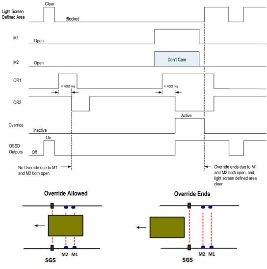
Figure 2. Muting Timing Diagram – L Configuration
