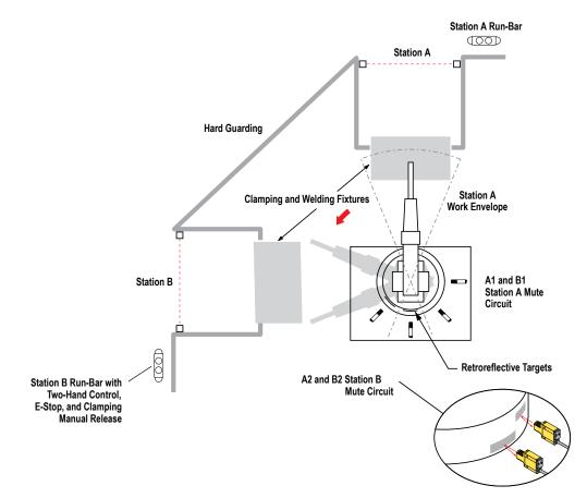
Figure 29. A robot load/unload application with two-station home-position muting, using polarized retroreflective photoelectrics as muting devices
